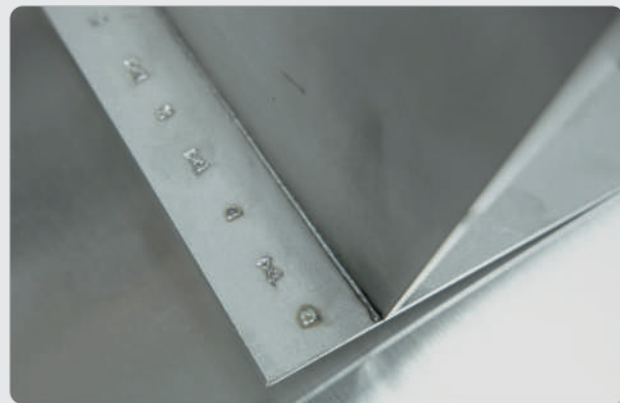
Welding of thin materials without added wire
