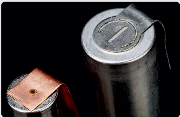
Welding of dissimilar metals
