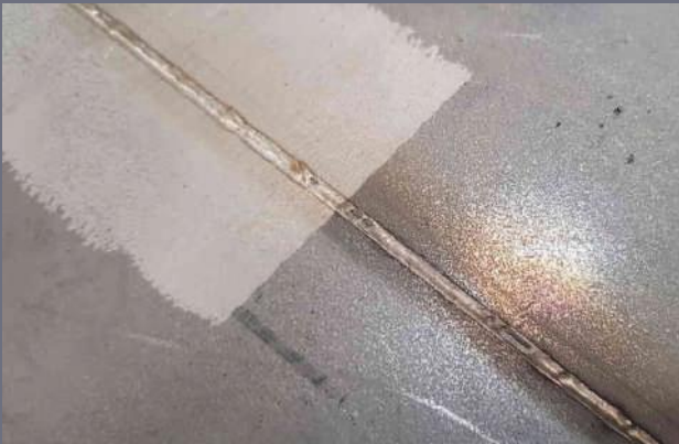
LASER WELD PROCESSED BY LASER CLEANING METHOD
