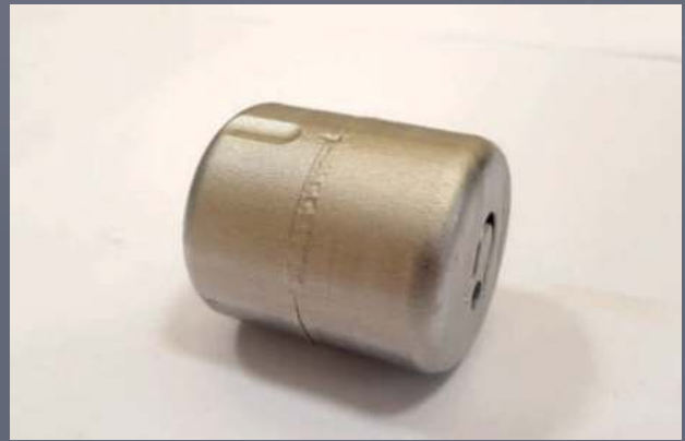
WELDING OF ROUND ALUMINIUM PIECE
