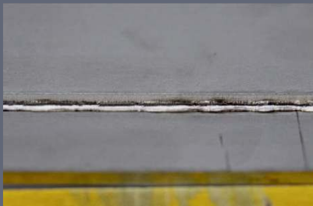
WELDING OF STEEL WITHOUT FILLER METAL
