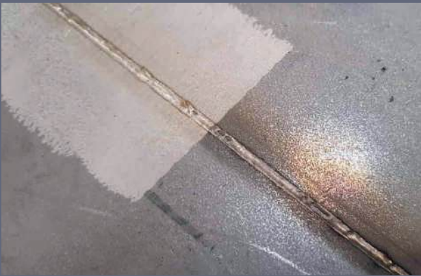
LASER WELD PROCESSED BY LASER CLEANING METHOD
