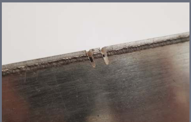
FIBER LASER WELD CUT ON ALUMINIUM
