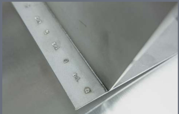
WELDING WITHOUT FILLER METAL FOR THIN MATERIALS
