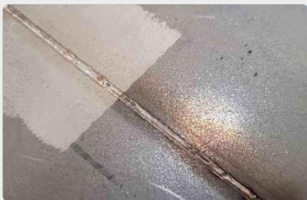
Oxidation cleaning before and after welding
