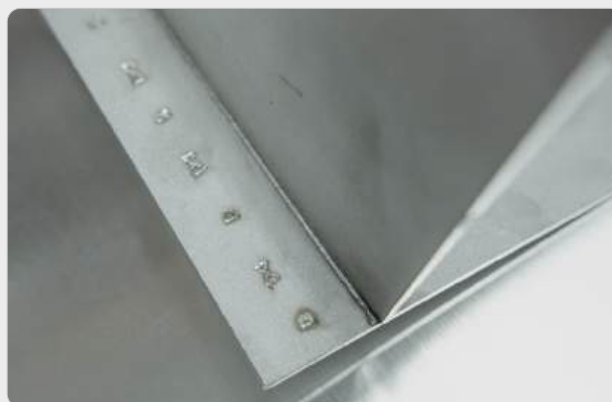
Welding of thin materials without added wire
